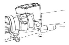
Please link the cable of control pad (B) to the display unit and link the display unit (A) to the EB-BUS cable.
