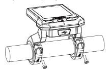
Open the clamp on the control pad and place it in the correct position, Using 1 X M3\*8 screw tighten the control pad onto the handlebar. Torque requirement: 1N.m.
